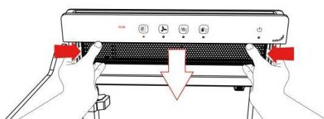
Detach filter housing (press the catches at the side)
