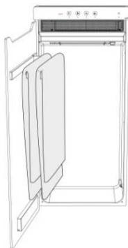
Remove the textiles that are blocking airways or the heated glass door (see Steps 2 to 4) and hang up the textiles tidily
