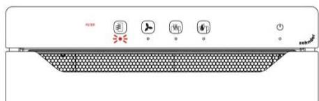
**FILTER** text appears and lights up continuously red. First indicator light on the left flashes white
