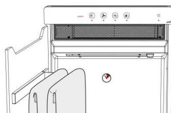
Wait 5 – 10 minutes with the door open to allow the unit to continue cooling down.
