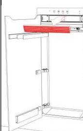
Carefully remove the filter housing
