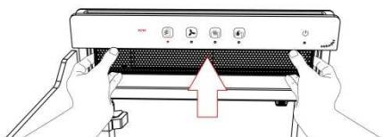
Refit the filter housing (so the catches engage)
